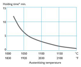
\* Holding time = time at austenitizing temperature after the tool is fully heated through.
